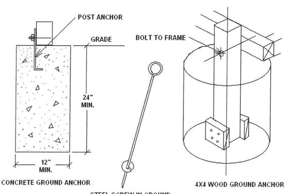
STEEL SCREW-IN GROUND ANCHOR (INSTALL PER MANUFACTURE INSTRUCTIONS)
